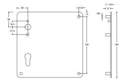
\* Observe drilling or milling dimensions for handle and WC mounting holes – please request the relevant mounting instruction!
