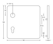
$^{\star\star}$  Observe drilling or milling dimension for handle hole Ø 25 mm!
